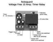
The Roboguard Timer Relay should be used when the distance from the HQ to the siren is greater than 10 metres.
